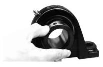
The inner ring of the bearing is locked to the shaft by a quarter-turn of the eccentric collar in the direction of shaft rotation. The collar is secured in place with a single setscrew.
